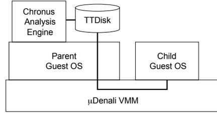
Figure 2: **Chronus Architecture:** During normal operation, disk writes are logged to a Time Travel Disk. During analysis, Chronus rolls back time and runs a user-provided software probe to test whether the system was in a correct state.
